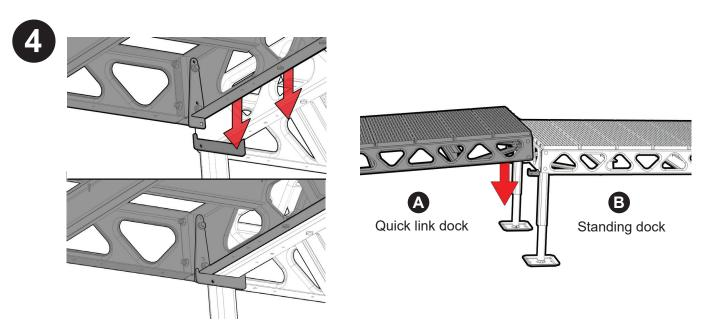
Decking can now be installed on your dock. After decking has been finished you may lower the quick link dock (A) onto the "L" shaped bracket (QLB1) of the existing standing dock.
