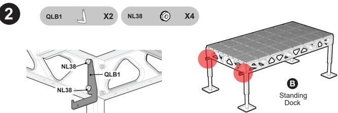
Position the "L" shaped bracket (QLB1) on **top of current locknuts**. Fasten the L-Bracket with locknuts (NL38). Repeat **Step 3** for opposite side of the dock.
