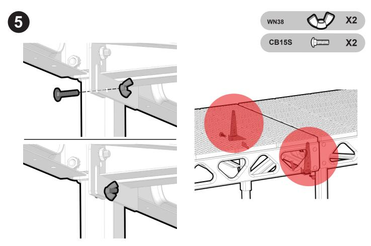
Align holes of both brackets and insert bolt (CB15S). Fasten bolt with wingnut (WN38). Repeat **Step 5** for the opposite side of the dock.
