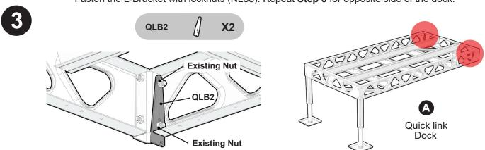
Remove the existing locknuts. Position the joining bracket (QLB2) on the bolts and fasten with existing nuts (See image above). Repeat **Step 2** for the opposite side of the dock.
