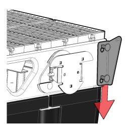
Attach the hinge cover bracket(HBR1) to the loosened carriage bolts at the end of the dock or ramp. Slide the hinge cover bracket(HBR1) down on the carriage bolts until they are seated in the narrow slots of the bracket.
