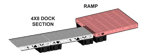
On dock configurations that transition between 4x8 and 8x8 docks ensure the hinge bracket is installed to the **4x8 section**.
