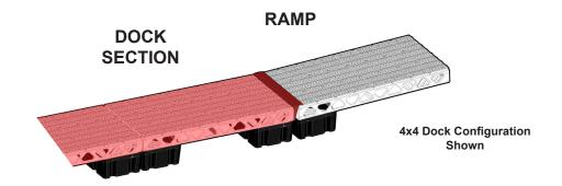
On dock systems that transition from same size docks (4x8 to 4x8 docks or 8x8 to 8x8 docks) ensure the hinge cover bracket is installed to the **dock section**.
