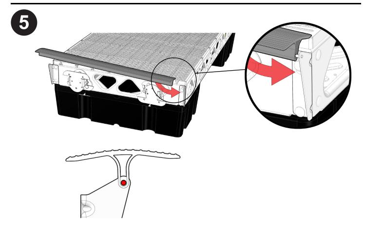
Position and slide the hinge cover onto the pin located at the top of the hinge cover bracket(HBR1).
