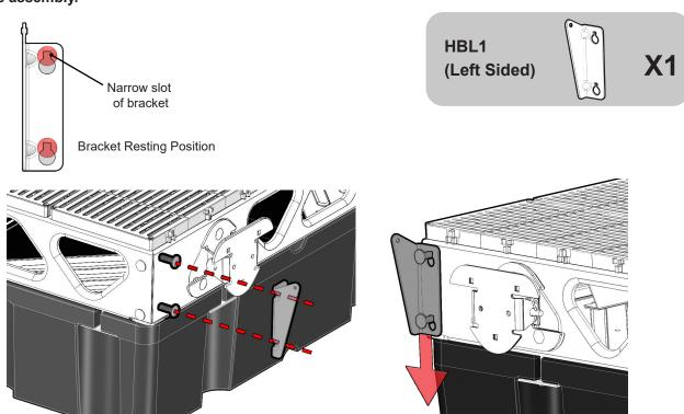
Attach the hinge cover bracket(HBL1) to the loosened carriage bolts at the end of the dock or ramp. Slide the hinge cover bracket(HBL1) down on the carriage bolts until they are seated in the narrow slots of the bracket.
