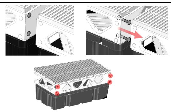
Using a socket/ratchet or box wrench, loosen carriage bolts on both dock or ramp that you will be attaching the hinge cover to (See image above for carriage bolt locations).
