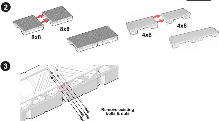
**PLEASE NOTE:** Some details such as decking has been removed to better illustrate assembly. **TIP:** Adjust dock height to align holes. Pry bar may help. Mallet or soft faced hammer may be needed to encourage bolts into place.
