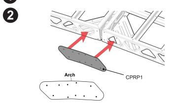
**PLEASE NOTE:** Connector (CPRP1) should have arch facing upwards. Two connected ramps will settle after the initial use to create a straight platform.
