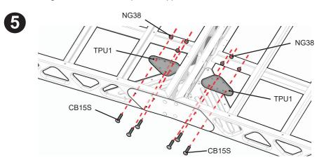
Attach Triangle Backing Plates(TPU1) using Bolts(CB15S) and Nuts (NG38). Do this for both Connector Plates(CPRP1).
