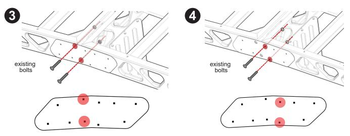
Undo 4 Carriage Bolts (3-1/2" long). Fasten Connector Plate (CPRP1) with existing 4 Bolts (CB15S), and Nuts (NG38). Handtighten at this time. Repeat on opposite side of dock.
