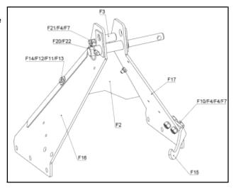
2 . Hung the assembled components according to the hanging installation diagram on the hood, install the suspension components of bolt hole and the gearbox bracket( F1 8 ) on the hood welded parts installation hole alignment, then install the lower hitch- R( F23 ) and lower hitch- L( F24 ) , install and tighten the bolts, flat washers and lock nuts in turn, and finally insert the lower hanging pin and lock pin (F25 and F20).
