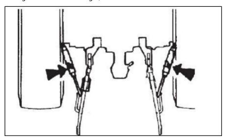
If the magnitude of the tractor towing arms is too narrow, adjust the left suspension pin inward as below:
