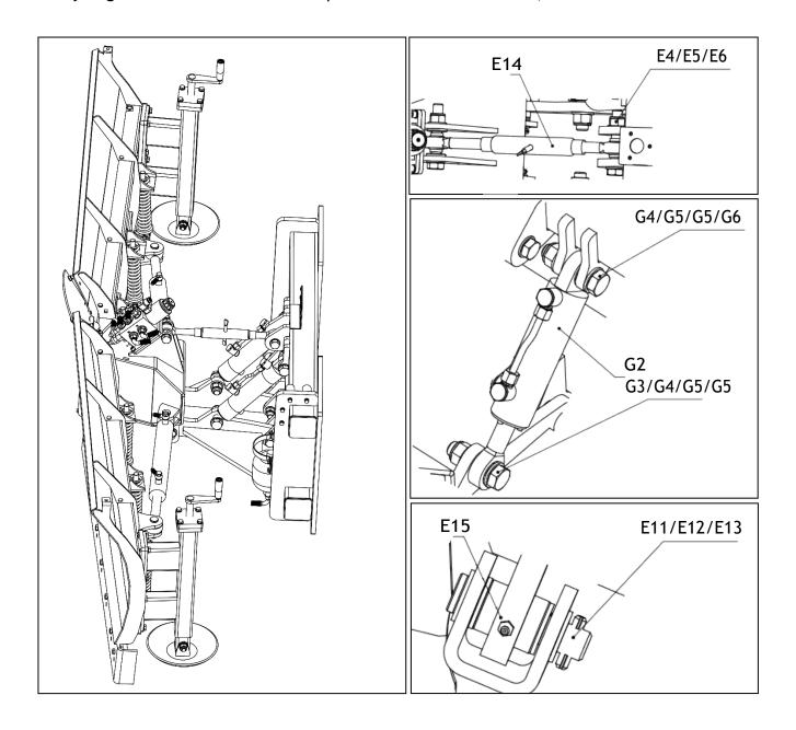
bolt (E5) with the washer (E4) and lock nut (E6) to tighten. The ring and lock nut are tightened. **Importance:** All bolts are locked in place without shaking.
