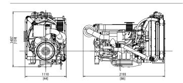
12.78 liter, in-line 6 cylinder - Constant engine speed Emission compliance: Stage V
