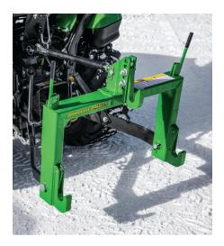
**iMatch<sup>™</sup> Quick-Hitch** Connect attachments and implements the easy way.
