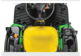
THE CONTROLS are located at hand next to the fenders and color-coded for easy identification
