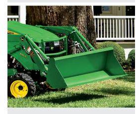
THE D120 LOADER is our most affordable loader option and is non-self-leveling (NSL). The lift capacity is 825 lbs at pivot (375 kg) with a max lift height of 71.2 in (1809 mm).
