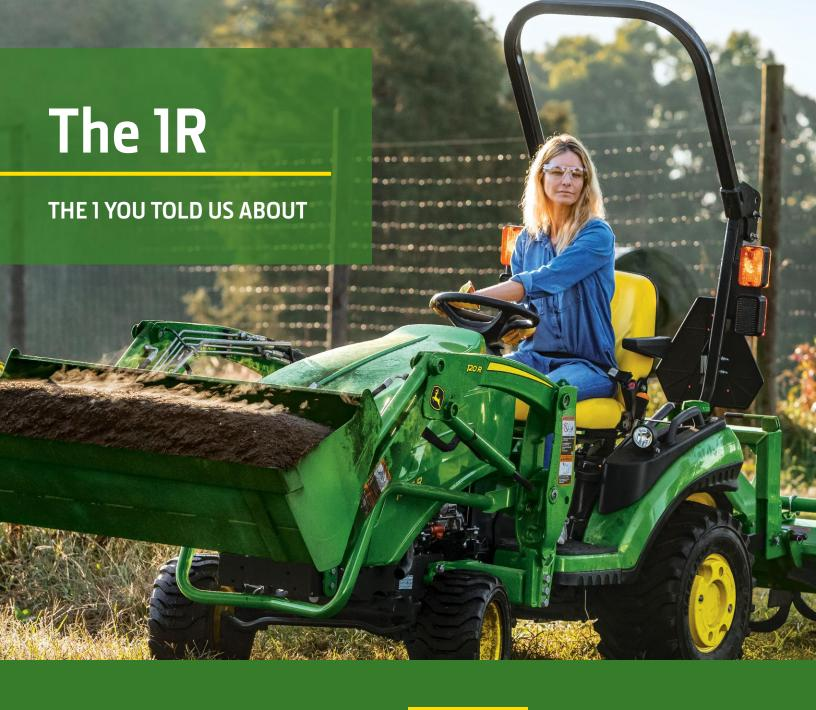
We asked sub-compact utility tractor owners during development, "what would the best small tractor look like to you?" The answer? This 1, the 1025R. The 1025R has a 23.9 HP<sup>2</sup> (17.8 kW), three-cylinder diesel engine that delivers responsive, efficient horsepower in just about any application. Everything from clearing a sidewalk or a driveway of snow to mowing an acre of lawn to digging out a water feature or drainage ditch.
