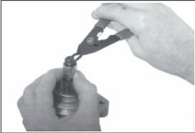
Figure 8-35. Removing Retaining Ring.
