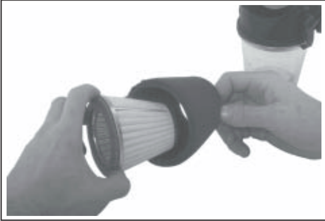
Figure 4-8. Removing Heavy-Duty Precleaner.
