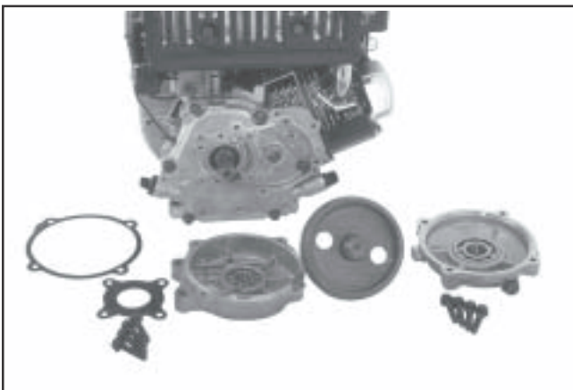
Figure 9-69. CS4, CS6 6:1 Reduction Assembly Components.
