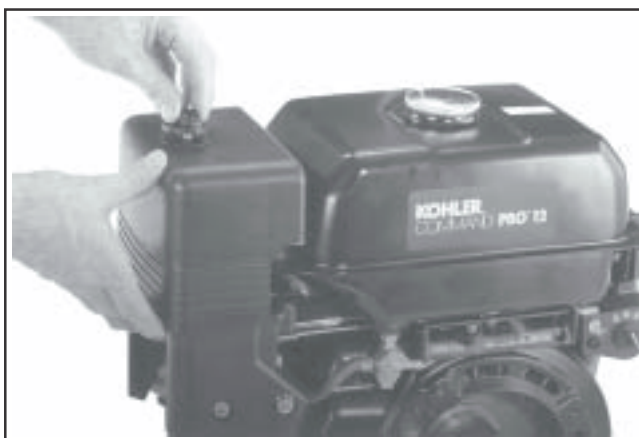
Figure 11-115. Installing Outer Air Cleaner Cover and Knob.
