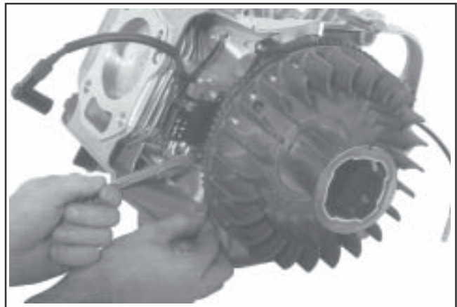
Figure 11-62. CS8.5-12. Setting Air Gap.
