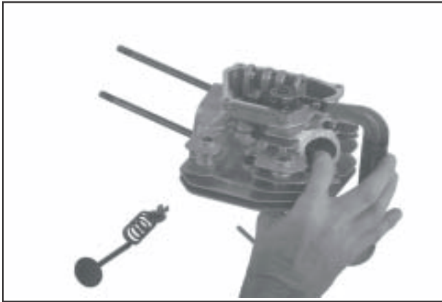
Figure 9-43. Disassembling Valve Assemblies.
