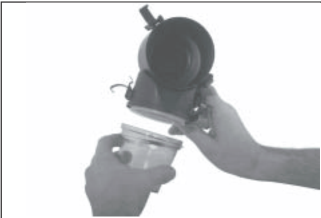
Figure 4-9. Removing Heavy-Duty Lower Chamber.
