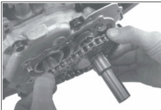
Figure 9-60. Removing Sprockets and Chain on CS4, CS6.
