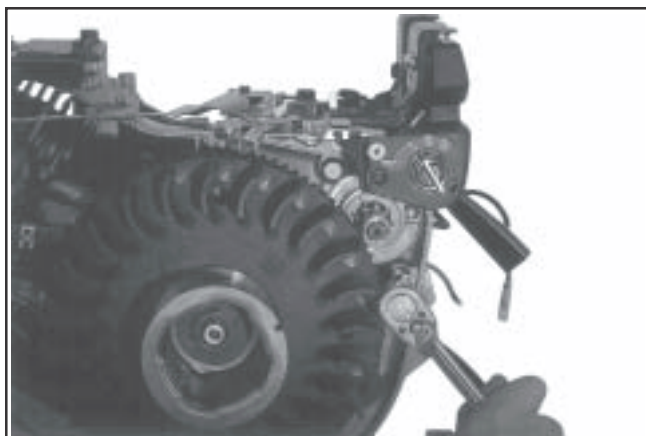
Figure 9-29. Removing Inertia Drive Starter Mounting Bolts.
