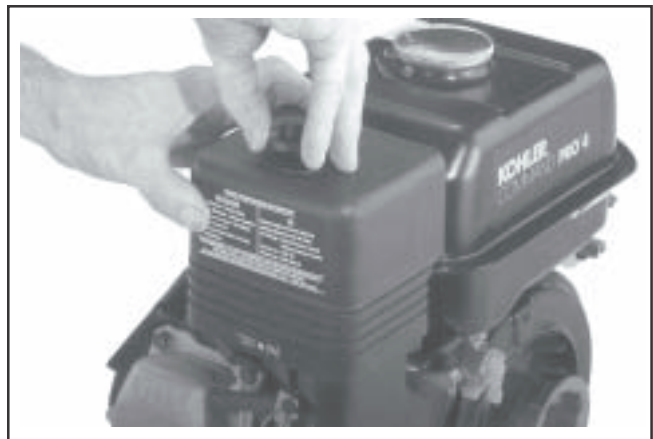
Figure 4-3. Removing Cover Knob Standard.
