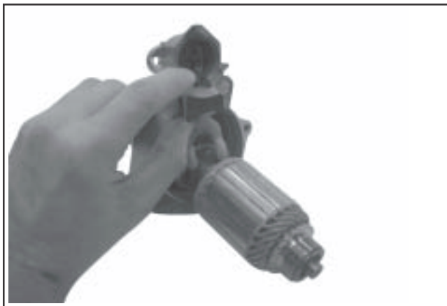
Figure 8-60. Removing Drive Lever and Armature.
