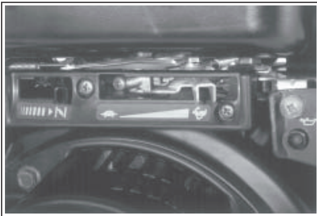
Figure 11-119. CS8.5 (spec. 92xxxx), CS10, CS12. High Speed Stop Screw.
