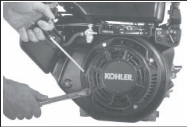
Figure 11-116. Engage Pawls and Torque Mounting Screws.
