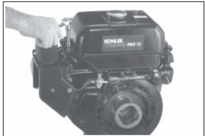
Figure 11-111. Tightening Fuel Tank Mounting Screws.
