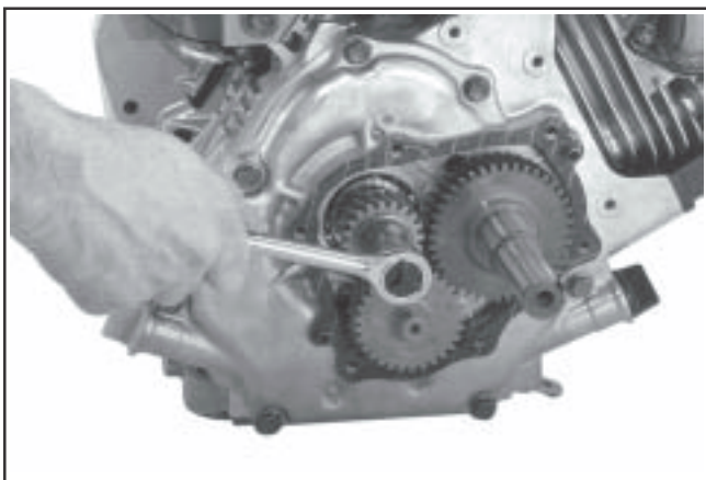
Figure 9-59. Removing Screw from Crankshaft on CS8.5-CS12.
