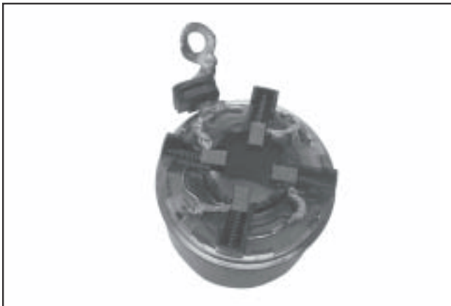
Figure 8-64. Mounting Brush Holder to Frame.
