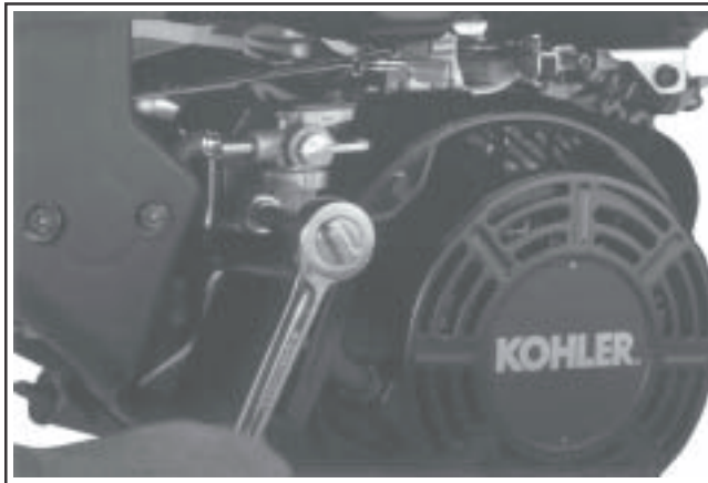
Figure 11-114. CS8.5 (spec. 95xxxx). Mounting Shut-Off Valve.
