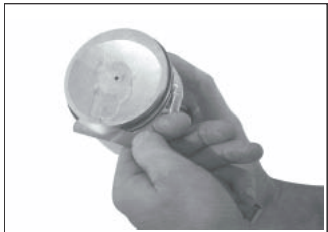
Figure 10-15. Measuring Piston Ring Side Clearance.
