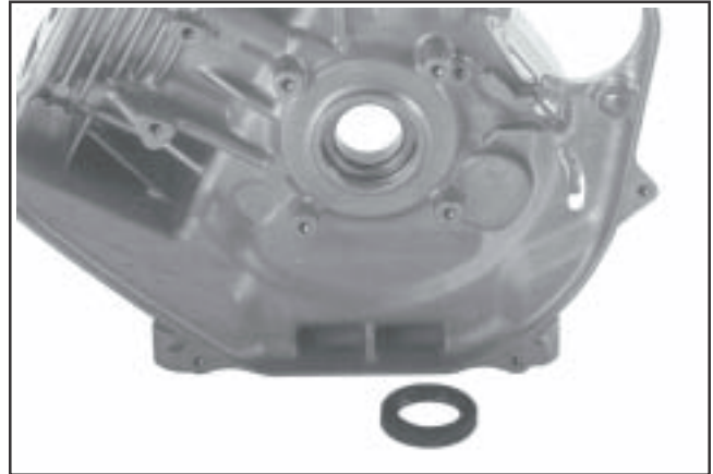
Figure 9-89. Oil Seal Removed.
