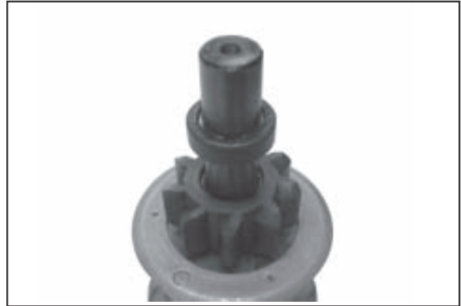
Figure 8-62. Lock Collar around Retaining Ring.
