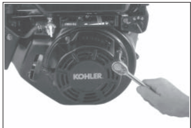
Figure 7-2. Installing Retractable Starter.
