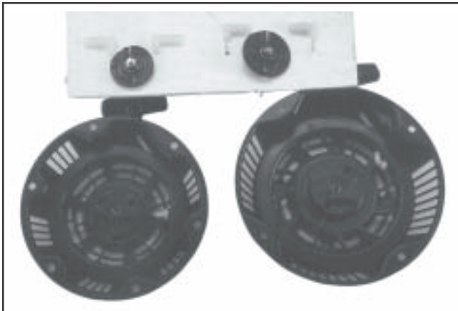
Figure 7-8. Retractable Starter Pawl Assembly Details.
