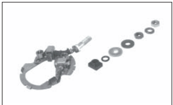
Figure 8-52. Brush Plate and Terminal Components.
