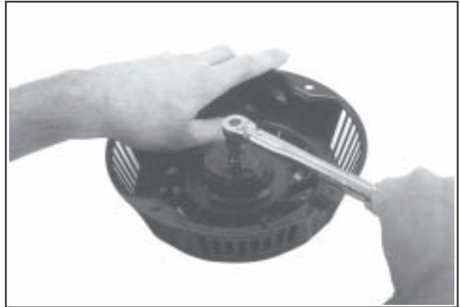
Figure 7-11. Torque Center Mounting Screw.
