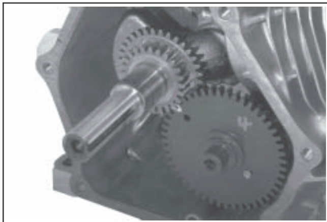
Figure 11-15. CS4, CS6. Aligning Crankshaft and Camshaft Timing Marks.
