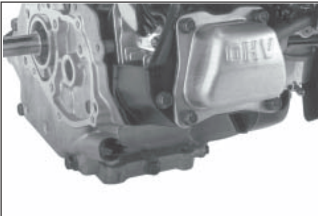
Figure 6-5. CS4, CS6 Left Oil Fill/Level Plug Location.
