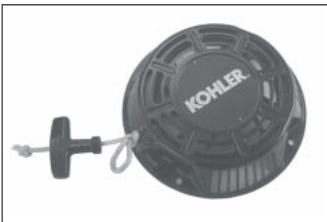
Figure 7-4. Removing Starter Handle.
