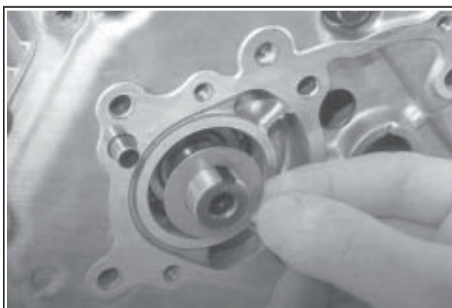
Figure 9-61. Thrust Washer Behind Crank Sprocket on CS4, CS6.
