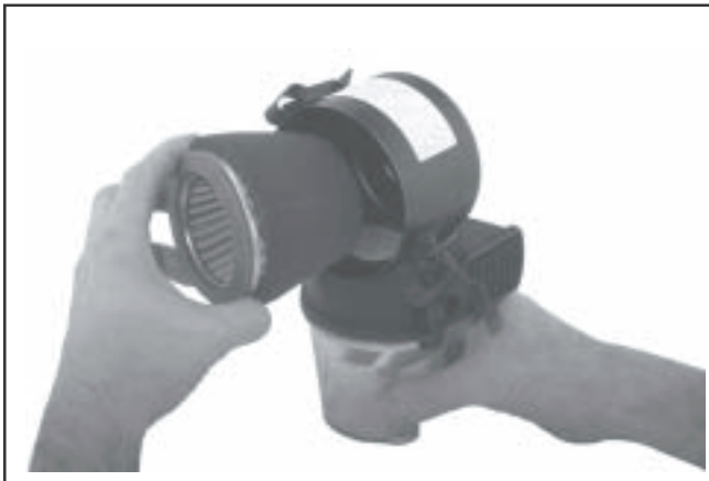
Figure 4-6. Heavy-Duty Element/Precleaner Assembly.
