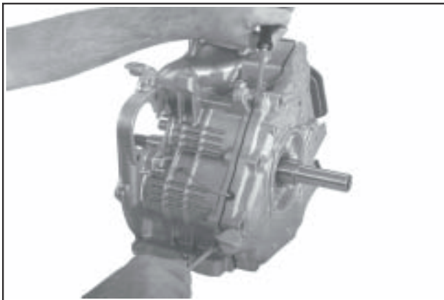
Figure 9-77. Separating Closure Plate From Crankcase.
