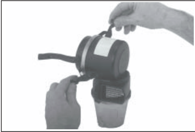
Figure 4-4. Unsnapping Heavy-Duty Latches.
