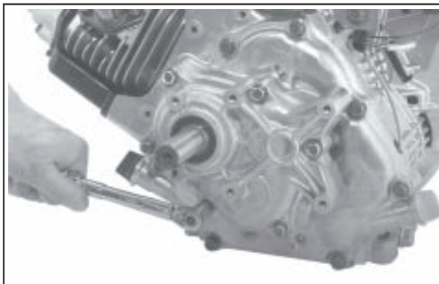
Figure 11-37. CS8.5-12. Torquing Cover Mounting Screws.
