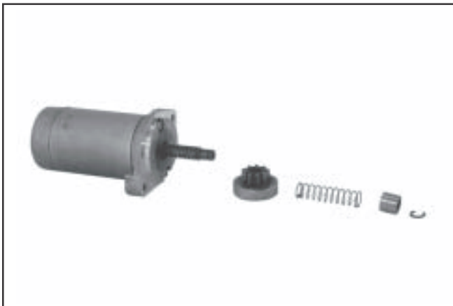
Figure 8-36. Disassembled Drive Components.
