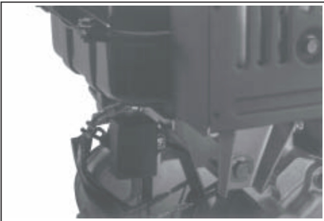
Figure 9-25. CS8.5 (spec. 95xxxx) Ground Lead Location.
