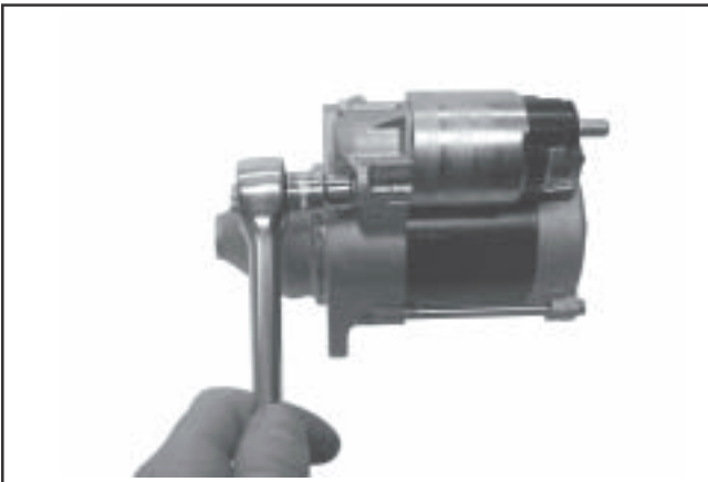
Figure 8-69. Installing Thru Bolts.
