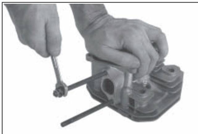
Figure 9-45. Removing Carburetor Mounting Studs.
