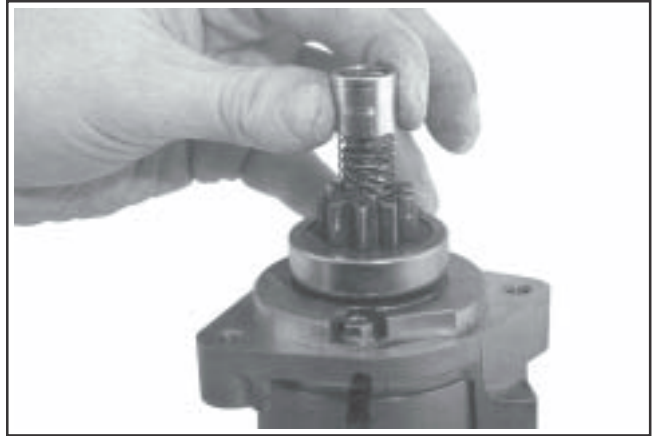
Figure 8-37. Installing Drive Components.
