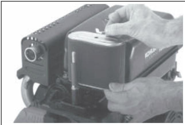
Figure 4-5. Standard Element/Precleaner Assembly.
