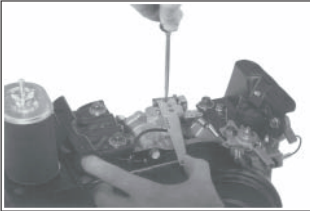
Figure 11-108. CS4, CS6. Adjusting Governor.
