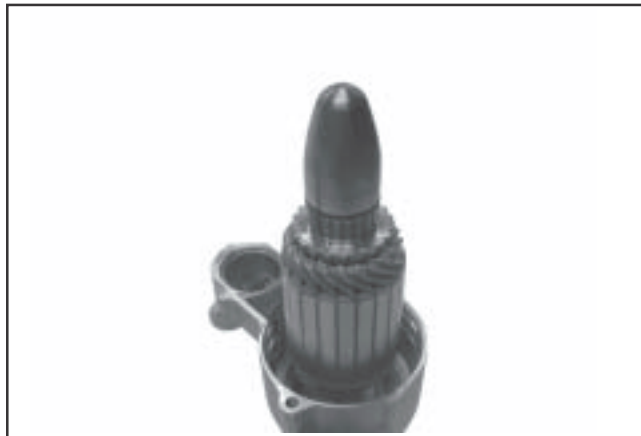
Figure 8-66. Tool on end of Armature.
