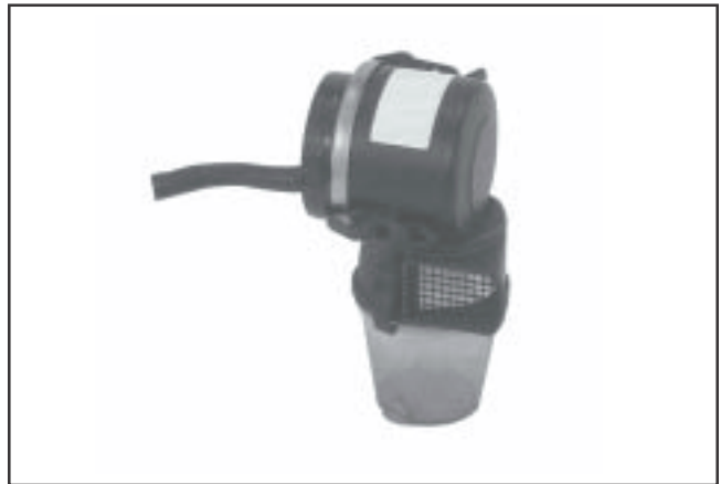
Figure 4-2. Heavy-Duty, Cyclonic Air Cleaner.
