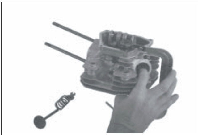
Figure 11-64. Installing Valves Using Valve Spring Compressor.
