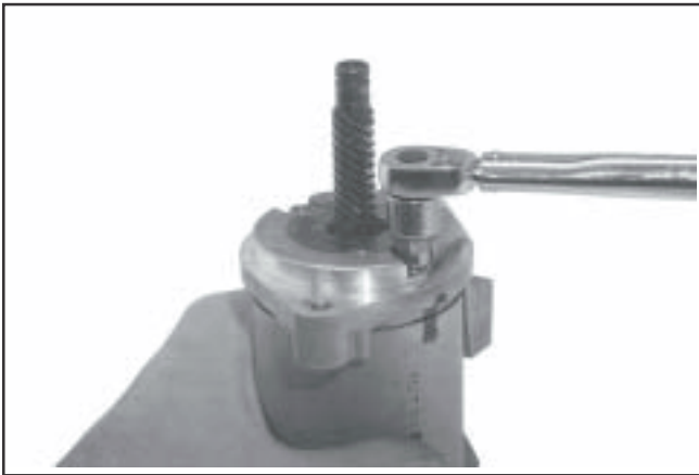
Figure 8-54. Torquing Thru Bolts.
