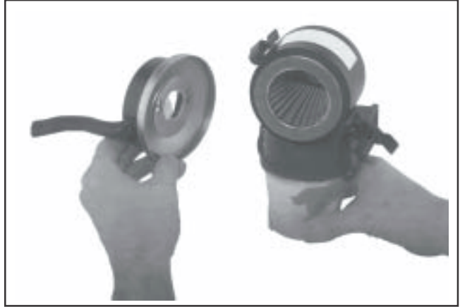
Figure 4-11. Installing Heavy-Duty Cover/Housing.
