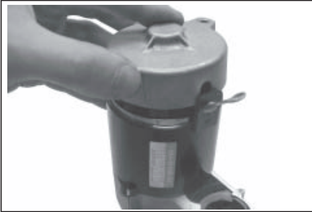
Figure 8-68. Installing End Cap.
