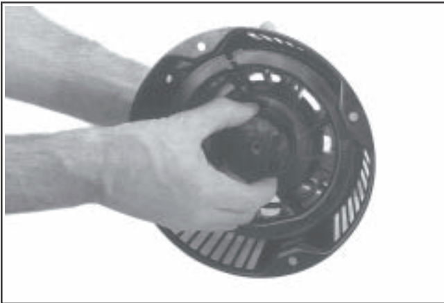
Figure 7-10. Assembling Starter Pulley to Housing.
