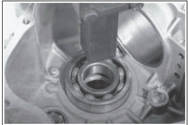
Figure 11-1. Installing Bearings Using a Press.
