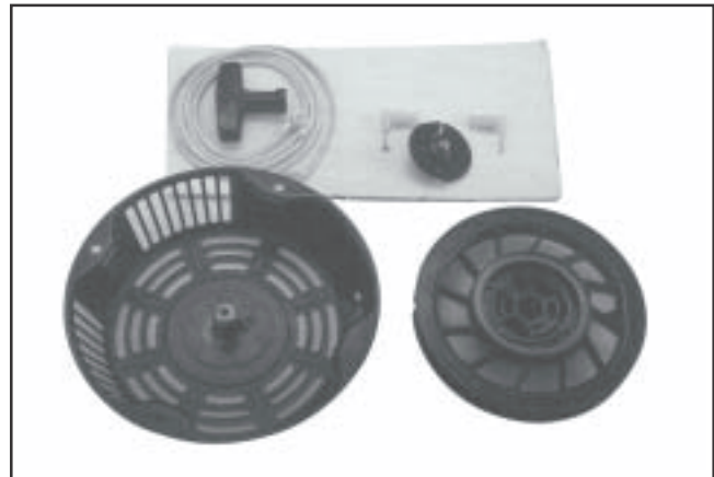
Figure 7-9. Disassembled Retractable Starter.
