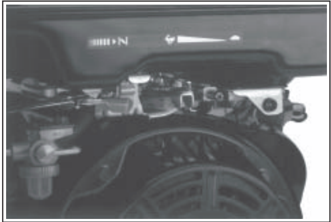
Figure 11-120. CS8.5 (spec. 95xxxx). High Speed Stop Screw.
