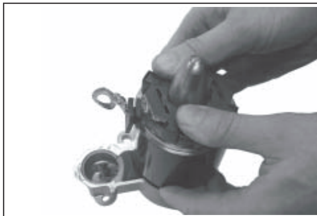
Figure 8-67. Installing Frame with Brush Plate Assembly.
