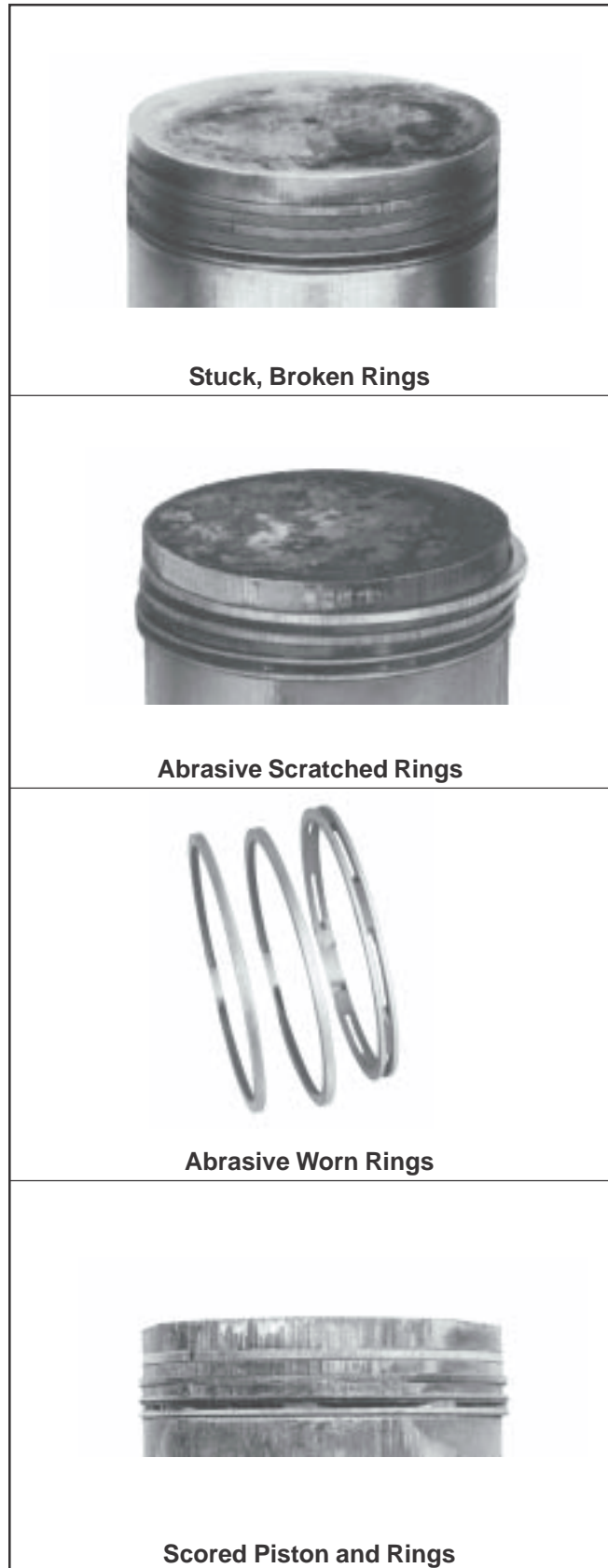
Figure 10-13. Common Types of Piston and Ring Damage.
