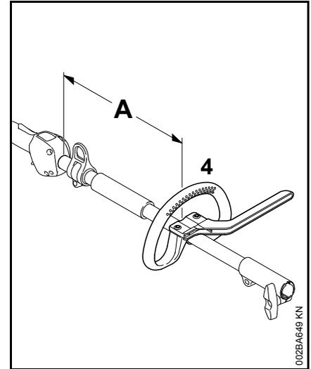
The loop handle can be adjusted to suit the height and reach of the operator and the application by changing distance (A).
