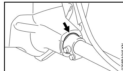
A vibration-absorbing rubber element is installed between the powerhead and the drive tube. Have it checked if there are signs of wear or a noticeable increase in vibration levels.
