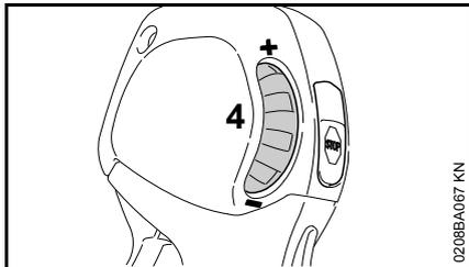
The throttle set wheel (4) enables the travel of the throttle trigger to be preset anywhere between idle and full throttle.
