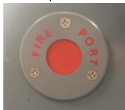
Fire port- located on the port side of the console
