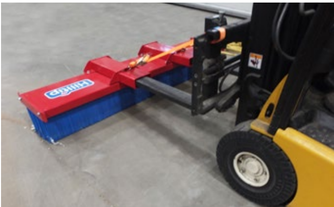
SweepAway™ with attachment for forklift
