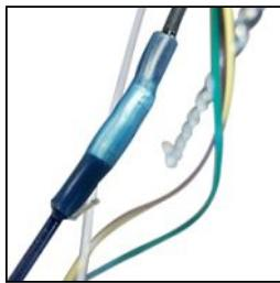
**Heat-Shrunk Sealed, Concealed Wiring**
