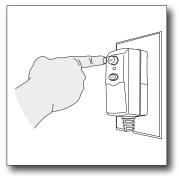
15. Plug machine into a grounded outlet, push reset button.
