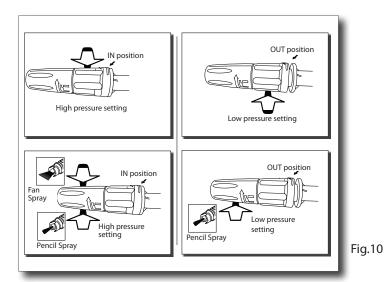
IN position for high pressure spray. Twist the nozzle counterclockwise until it stops and gap is closed. OUT position for low pressure spray for detergent function. Twist the nozzle clockwise until it stops and gap is open.
