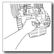
Pull clear siphoning tube through cap so it will draw detergent from bottom of tank.
