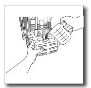
Fill detergent tank (page 11). Do NOT use thick detergent as it can clog the power washer.
