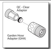
14. Clear QC adapter attaches to power washer, GHA attaches to garden hose.
