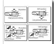
8. The adjustable spray nozzle had has two (2) positions: •IN position for high pressure spray. Designed to use for cleaning and allowing spray to be adjusted. • OUT position for low pressure spray for detergent function. Spray needs to be set with fan blades in the "pencil stream" position to assure the detergent is not restricted.
