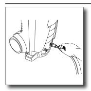
Snap the GHA onto the QC adapter. To remove pull back on the collar and pull off.
