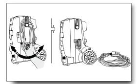
3. Swivel bottom cord hook right or left to easily remove the power cord.
