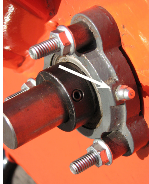
Figure 5.13, Chute Side Bearing Zerk
