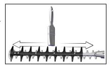
Wipe excess oil from the blade before putting the unit back in service. 4.
