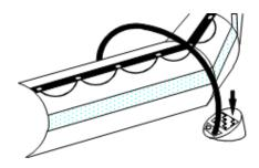
**4º/** Inflate the inflatable tube, starting with the first compartment (a) at the bow, to 200 mb pressure.
