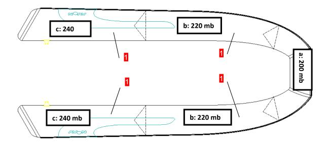
**NOTE:** A slight loss of air is normal before the cap is screwed on. <u>Only the plugs provide final airtightness.</u>
