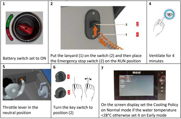
\* If the pilot falls overboard, immediately stopping the engine considerably reduces the risks of serious or fatal injury caused by being run over by the boat. Always couple the two ends of the emergency stop switch correctly.
