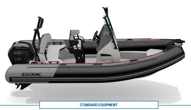
HULL & DECK: 1 Bow Bitt / 2 Aft Cleats, 1 Bow D Ring / 2 Towing Rings, 2 Bailers, Built-in Fuel Tank 100L, Fairleads, GRP Deep V-Hull, Lockable Mooring Storage, Ski & Wakeboard Locker, Tilting Console.
