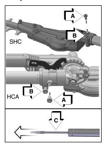
Pull the drive shaft (C) from the housing, wipe clean, then apply 15 ml (0.5 oz.) of grease.
