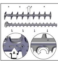
Use new lock nuts each time blade guard is installed. See dealer for correct nuts.
