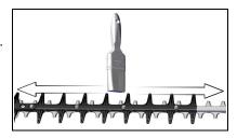
Wipe excess oil from the blade before putting the unit back in service. 4.
