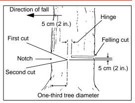
about 5 cm (2 in.) will act as a hinge when the tree falls, guiding it in the desired direction. When the tree starts to fall, kill the engine, place the saw on the ground and make your retreat quickly.
