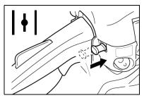
Note: Do not increase engine speed while chain brake is locked. Severe brake damage will result.
