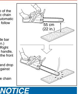
When checking the operation of the automatic chain brake, use a soft surface substance like wood to absorb the impact so the chain is not damaged.
