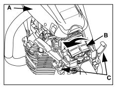
6. Install air filter and cylinder cover, engage latches.
