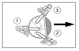
final cut is made by drawing the saw forward in the cut to reach the hinge.
