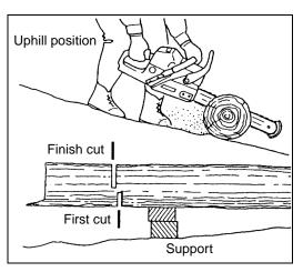
trunk will weaken at the point where you make the cut unless the tree is lying on perfectly flat ground or supported as shown. If you make the cut with the tree on the ground, don't let the saw's chain dig into the earth; it is harmful for the saw, and you stand a good chance of being struck by flying debris.
