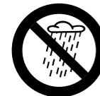
The drive motor is not waterproof. Never work with the machine in the rain or in wet or very damp locations.
