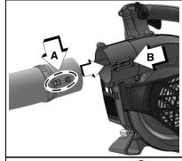
Do not assemble the opposite end of the upper blower pipe to the fan case.
