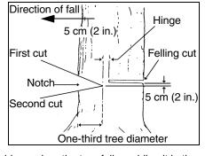
cut about 5 cm (2 in.) will act as a hinge when the tree falls, guiding it in the desired direction. When the tree starts to fall, kill the engine, place the saw on the ground and make your retreat quickly.
