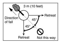
Begin the cut on the side to which the tree is to fall. Cut a notch about 1/3 of the way into the tree. The position of this notch is important since the tree will try to fall "into" the notch. The felling cut is made on the side opposite the notch and at a level about 5 cm (2 in.) above the bottom of the notch. Do not try to cut through to the notch with the felling cut. The remaining wood between the notch cut and felling
