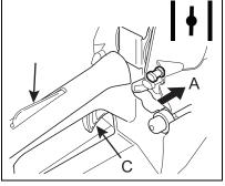
Note: Do not pull starter rope out to the maximum possible position. Do not allow recoil handle to snap back against the case. If engine does not start after 5 pulls, repeat instructions. Do not increase engine speed while chain brake is locked. Severe brake damage will result.
