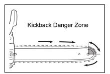
thumbs and fingers encircling the chain saw handles. A firm grip will help you reduce kickback and maintain control of the saw. Don't let go.
