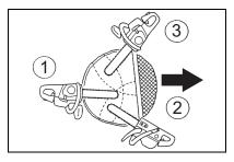
cut is made by drawing the saw forward in the cut to reach the hinge.
