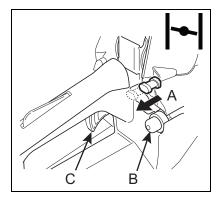
Securely hold the chain saw and pull starter handle several times until first starting sound.
