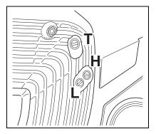
This engine has been factory adjusted to maintain satisfactory starting and durability performance up to 1,100 feet above sea level (ASL) (96.0 kPa). To maintain proper engine operation above 1,100 feet ASL the carburetor <u>may</u> need to be adjusted by an authorized service dealer.
