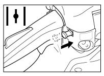
9 Pull starter handle to start the engine.
