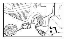
Do not damage fuel line while removing Fuel Filter (A) from tank.
