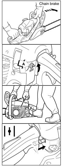
Note: Do not increase engine speed while chain brake is locked. Severe brake damage will result.
