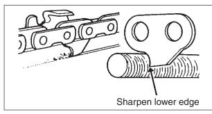
Important points for proper maintenance of saw chain:
