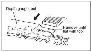
Place the depth gauge tool firmly on guide bar so that depth gauge protrudes. Then file top of depth gauge with the flat file until flat with top of the depth gauge tool.
