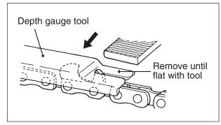
Place the depth gauge tool firmly on guide bar so that depth gauge protrudes.
