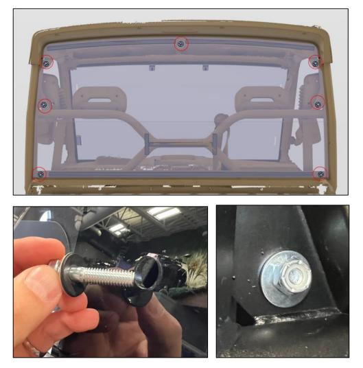
c) Tighten so that the gasket is fully pressed against the frame. Do not overtightened!
