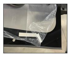
c) Remove approximately 6 inches of the liner on the gasket
