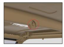
b) Remove protective layer along the contour of the back windshield
