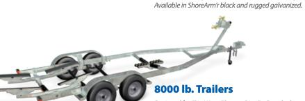
Designed for "Big Water" boats, this 3"x5" steel tube frame trailer is as tough as they come. They feature a heavy-duty uni-frame construction, dual axle disc brakes, heavy duty winchpost with double roller bow stop and solid aluminum fenders. Available in ShoreArm'r black and ruaged galvanized in roller or bunk.
