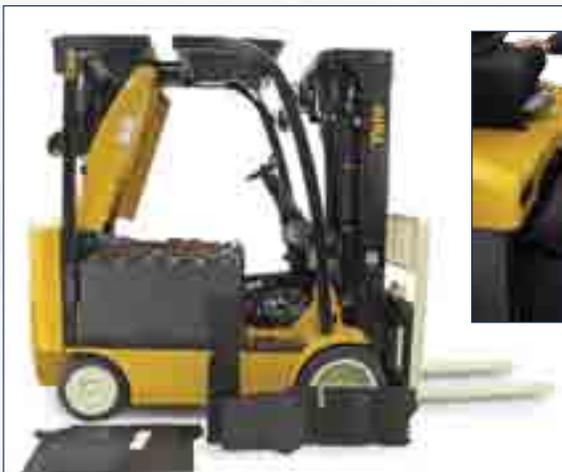
Two-piece floor plate allows for quick and easy service access. Removable floor plate side panels provide additional entry to key components.
