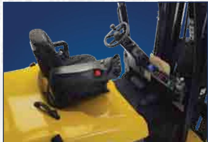
The location of the multifunction display provides maximum forward visibility and ease of operation. The multifunction display is located within easy reach of the operator or service technician for quick access to truck functions, diagnostics and troubleshooting without obstructing the forward view of the operator.
