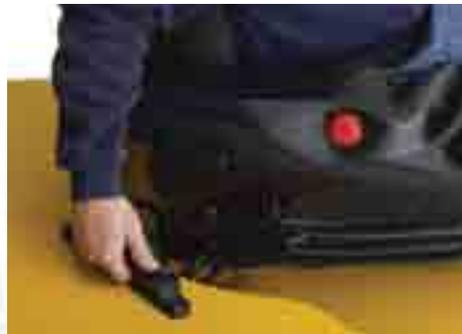
Rear driving comfort has been enhanced with a convenient optional rear drive handle with horn button. The rear drive handle, in conjunction with the optional swivel seat, creates a comfortable, secure reverse driving position. Non-cinching seat belts provide superior operator comfort.
