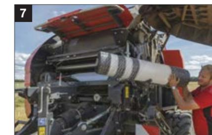
Support brackets for easy loading of the net roll
