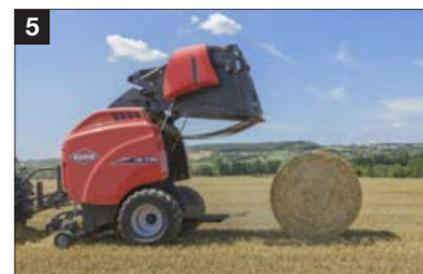
Within 4 seconds the bale is ejected and the tailgate is closed again
