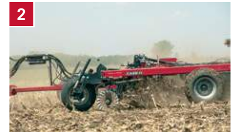
Disk Gang Depth: slice, cut and bury residue
