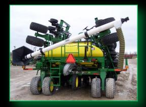
\*15' DESIGNED FOR MOST 15' NO-TILL/MIN-TILL DRILLS. \*AVAILABLE WITH BRISTLE, CUPPED STEEL OR 5" CUPPED PLASTIC FLIGHTING.
