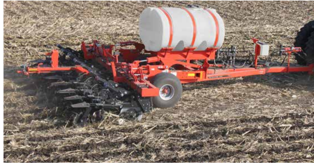
Gladiator 1210 pull-type models are all available with either 6-ton or 9-ton dry fertilizer tanks or a 1000 gallon liquid tank mounted on the chassis.
