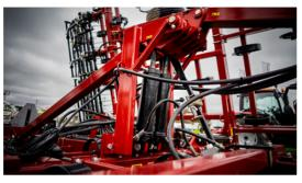
HYDRAULIC SELF-LEVELING FRAME The self-leveling frame sections of Salford cultivators follow ground contours exceptionally well. The unique frame design allows cultivators to remain level front to back and section to section as the machine follows ground undulations, providing reliable results in varying conditions.
