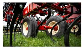
TANDEM AXLES Found on all Salford cultivators' mainframe, primary wing, and secondary wings. The tandems ensure that shovels on each cultivator section run at even depth as the cultivator crosses uneven ground, providing exceptionally consistent results.
