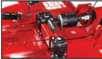
Shields over all cross shafts fold conveniently out of the way to allow quick access to clutch or universal joints.
