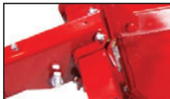
Wheel axles are attached by heavy duty pivot pins with replaceable bushings that extend through the cutter strongbacks. This dependable mounting arrangement provides extra strength and less pivot pin wear.
