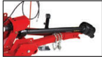
A wide angle, constant velocity driveshaft on pull models relieves the PTO working angle. This reduces vibration and allows smoother cutting in sharp turns.
