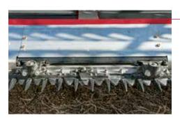
■ Knife heads, spline blocks, knife arms and hardware have been substantially beefed up to improve reliability and durability. More robust knife heads include a factory-assembled and lubed knife arm and head vertically mounted, allowing adjustments as required to obtain the proper gearbox-to-cutterbar spacing.
