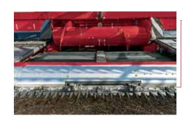
A seed saver channel along the bottom of the draper belt smoothly pulls grain into the combine, saving up to 3% more grain so no seed is left behind.
