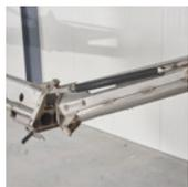
Spring loaded tip breakaway and mid boom shear bolt
