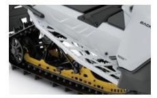
**4 Deep-snow running boards** Massive, strategically shaped openings keep the boards clear. A tall extruded edge adds stiffness and has aggressive boot grips.
