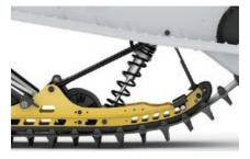
2 High-quality HPG shock package Extremely capable high-pressure gas shocks by KYB.<sup>†</sup>
