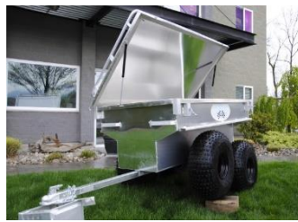
Gas shocks for easy lift on optional lid
