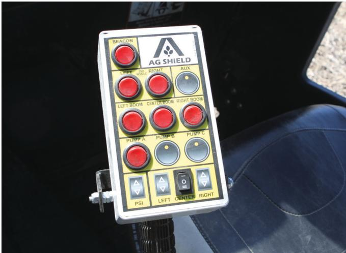
Integrated in-cab controls for all sprayer functions. Optional rate controller monitors vehicle speed and changes rate accordingly.
