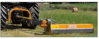
The gearbox position located outside of the transmission cover allows greater off-set of the flail head reducing the Pto shaft angle in work.
