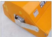
Rotor internal sealed bearings.
