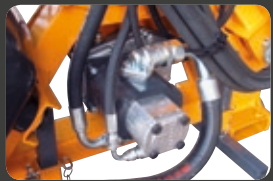
Cast iron hydraulic rotor pump group 3
