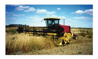
Lighter weight reels require less horsepower and lower drive loads.
