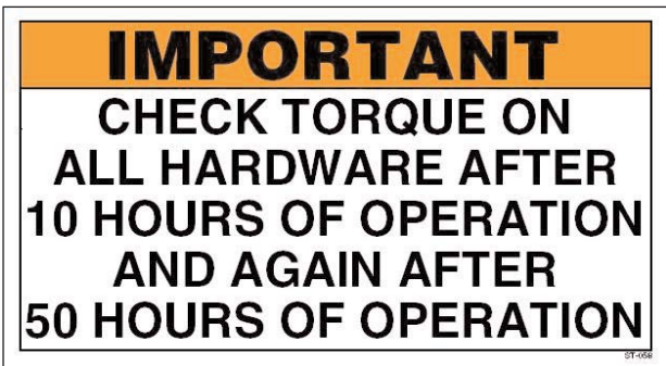
ST-058 Check Hardware Torque
