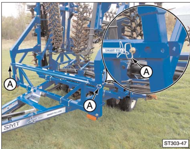
(A) Lock Pins with Hitch Clips (enlargement shows the lock pin in the storage location).
