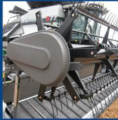
HCC's Flip Reel Kit is designed to prevent crops from wrapping around bat tubes and offers the durability needed to harvest tough crops including canola.
