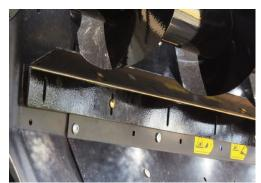
ANGLED STRIPPER BAR Our patented Angled Stripper Bar comes with each auger kit. It is designed to deflect crop into the auger flighting, promoting smooth and fast flow with less wrapping than competitors.
