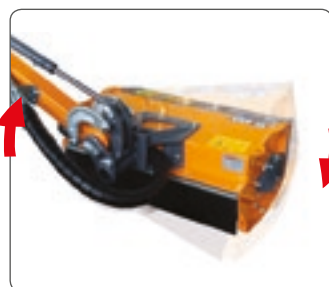
Sistema Floating. Floating head system.
