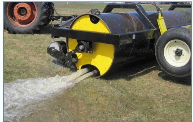
FIGURE 25 WATER DRAINING BY GRAVITY
