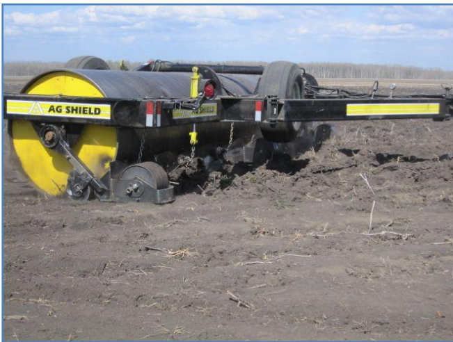
FIGURE 16 END GAUGING WHEEL SINKING INTO PLOUGHED GROUND
