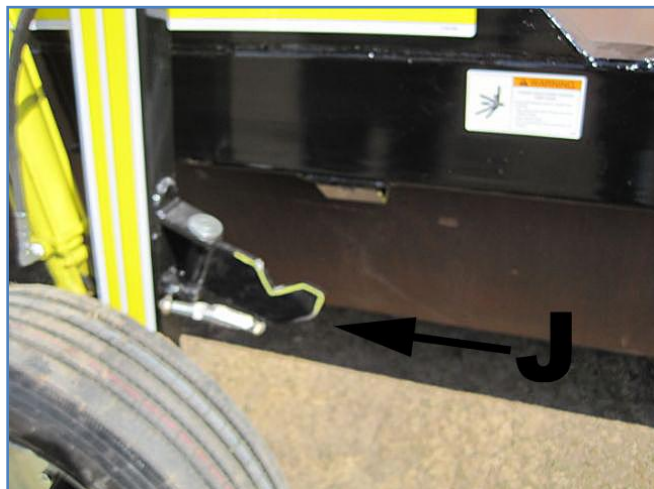
FIGURE 12 TRANSPORT LOCK FIELD POSITION
