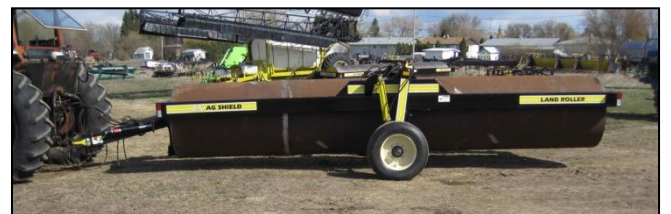
FIGURE 8 ROLLER BALANCED FOR PIVOT FOLD
