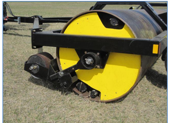
FIGURE 21 BLADE RAISED FOR TRANSPORT, CLEAR STONE, OR DUMP SOD
