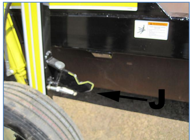
FIGURE 7 TRANSPORT LOCK FIELD POSITION
