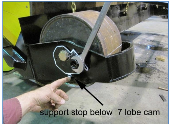
FIGURE 17 SUPPORT STOP AND ADJUST CAM
