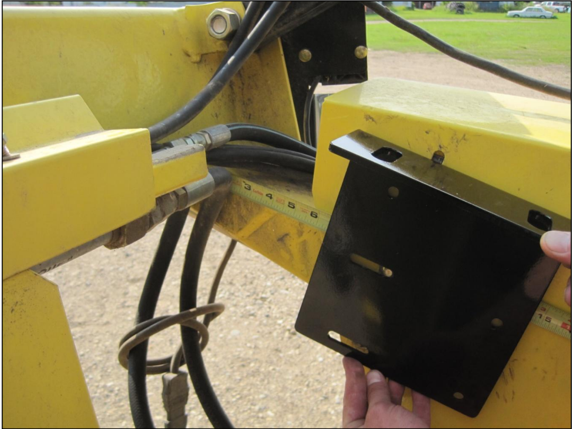
FIGURE 4 LEFT HAND MOUNT READY TO MARK HOLES
